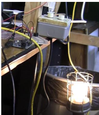
Figure 8. Incandescent light visualisation. The lightbulb’s luminescence corresponds to CO2 data from a Timestream.
