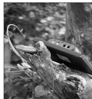
Figure 4. Mobile server and sensor collecting data in a tree for a short experiment in a Brazilian forest.
