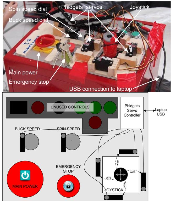
**Figure 3.** Broncomatic Controller and system diagram
